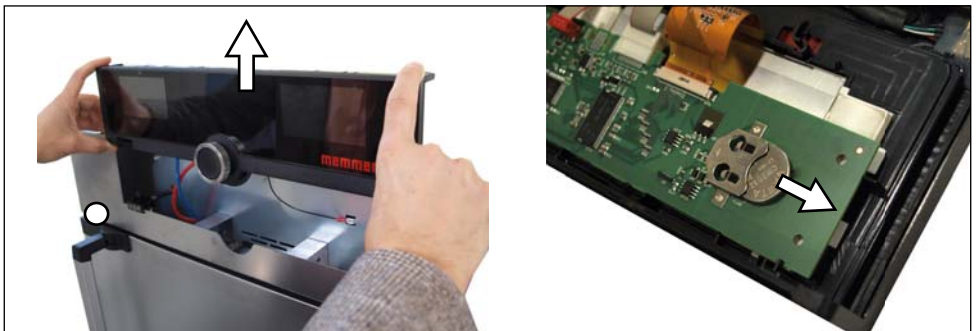
Fig. 31 Removing the lithium battery
